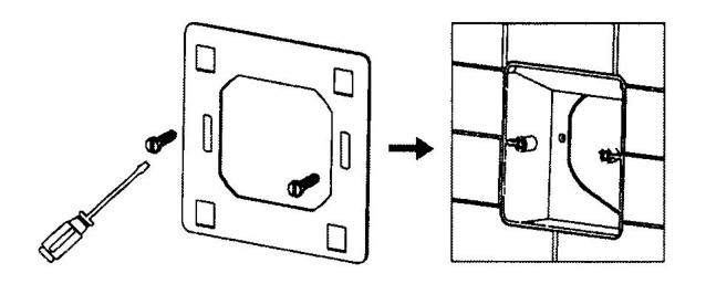
2 After connect wires (see right diagram), the themostat mounte on the backing plate.
