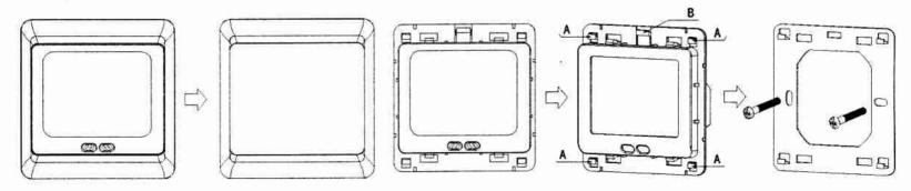
Step 1: Separate the Polycarbonate Bezel unit from the LCD screen.
